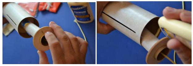
Slide in the motor mount tube until just the lower centering ring is sticking out. Spread glue in the body tube below the fin slots. Keep the glue off of the motor mount. Align the mark on the lower centering ring between two fin slots.
