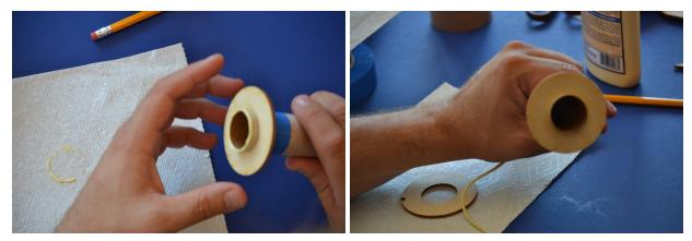
Twist on the centering ring until it reaches the tape, and clean any excess glue that has spread out. It is important to make sure there is no glue inside the motor mount. Allow the glue to set before moving on.
