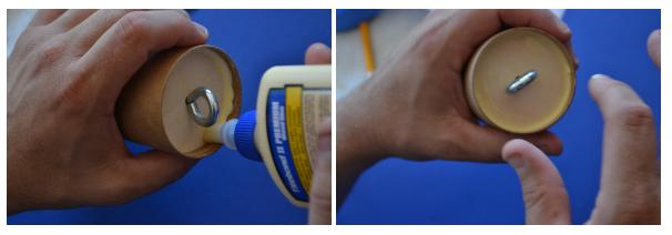
Add and spread glue to the corner of the bulkhead and the coupler. This fillet provides a better bond, especially helping when the shock cord will be tugging on the bulkhead in this direction in flight.
