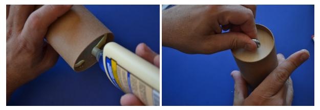
Glue the bulkhead into one end of the coupler by spreading glue on both surfaces and twisting into place. Position the bulkhead so that there is  $\frac{1}{4}$ - $\frac{1}{8}$  of an inch of coupler exposed.
