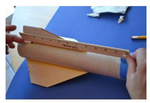
Before the glue sets, double check that both launch lugs are aligned.
