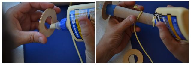
Spread glue to the inside of the centering ring and onto the motor mount tube at the mark.
