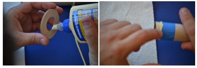
Remove the unnotched centering ring from the motor mount, and spread glue on the inside of the ring and the outside of the motor mount where the ring will go.
