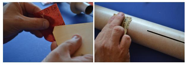
Test fit each fin in the body tube slots, and sand as needed, the fins should slide in snugly. Lightly sand the edge of each fin and the body tube above each fin slot. Again you are only looking to remove the shine from the cardboard tube.
