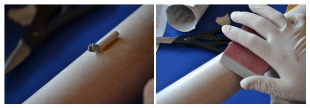
Tightly roll up newspaper and slide it into the launch lugs. Lightly sand the shiny coating off of the body tube to make paint adhere better. If painting the nose cone, lightly sand and use a paint that will adhere to plastic.
