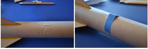
Using the mark made earlier, glue on the other launch lug, and use tape to hold it while the glue dries.
